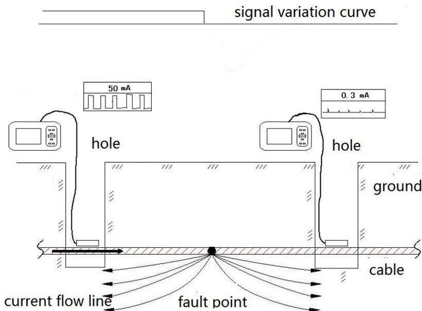
3.2.4 HV signal rod Fig.8 Step voltage pinpointing reference pinpointing
