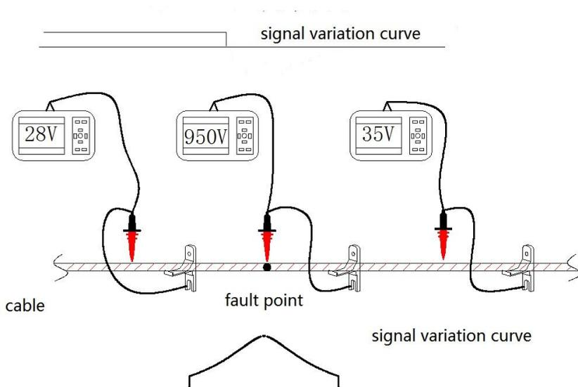
TI Fig.10 HV rod pinpointing section diagram ' CO.,LTD.
