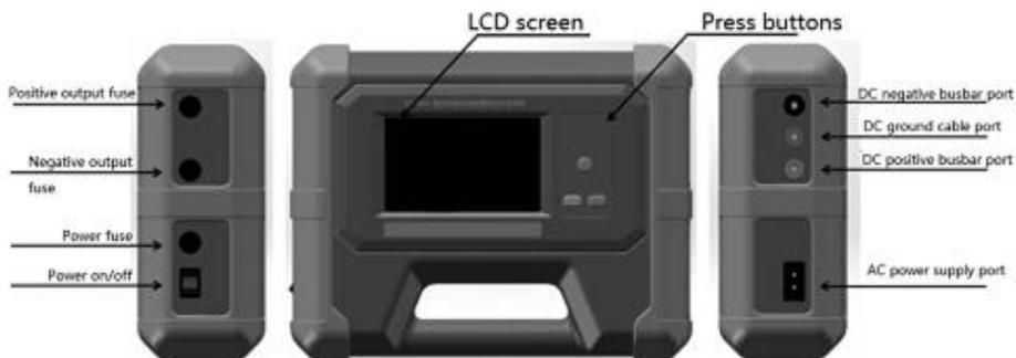
Fig.1 Transmitter appearance
