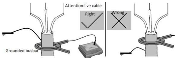
Fig.3.6 Clamp coupling method 1 (to clamp the cable)
