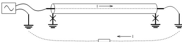
Loose the sheath of the both ends of the cable, also disconnect the earthing of Null line and Grounding line. Clamp one good conductor with the RED CLIP , and clamp the grounding rod with BLACK CLIP, connect the other end of the cable conductor to the grounding rod. At the cable opposite end, connect the core line with the grounding rod insert in the earth.
