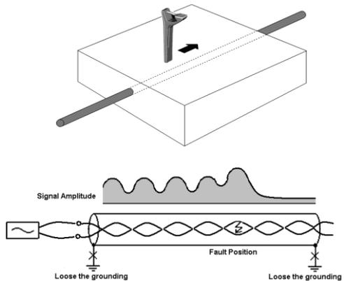
Fig.7.1 A frame fault locating process
