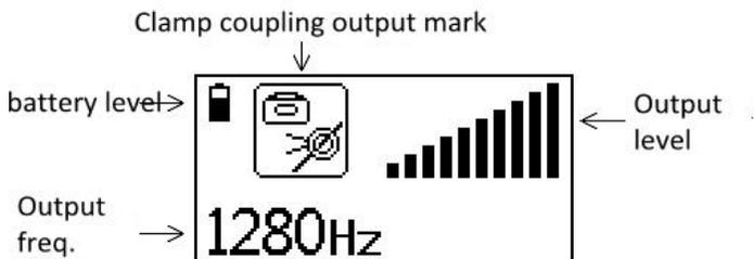
Fig.2.8 Clamp coupling output interface
