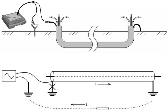
Fig.3.2 Sheath-Earth Method
