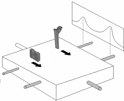
move simultaneously at the direction perpendicular to the cable/pipe. When the Transmitter passes the cable/pipe, the signal will be inducted into the pipe and the Receiver will receive signal. Observe the receiver responding and mark on the ground when peak responding above the pipe. Refer Fig. 4.8
