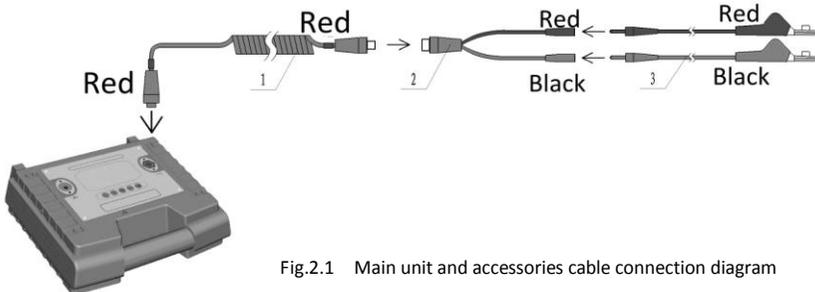
Fig.2.1 Main unit and accessories cable connection diagram
