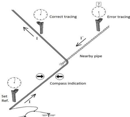
Fig.4.6 Intelligent tracing demo.
