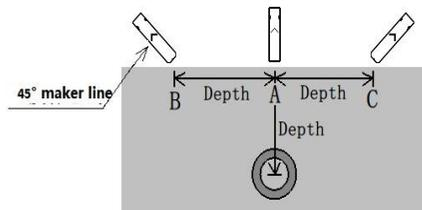
Fig.4.13 45% null manual depth measurement
