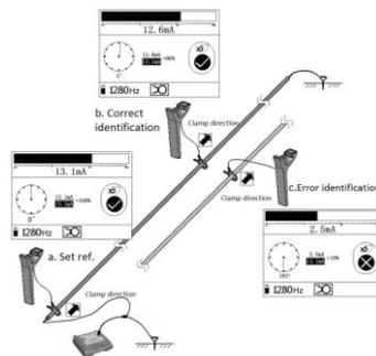
Fig.5.3 Clamp identification process
