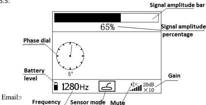
Fig.5.5 Sensor identification mode interface
