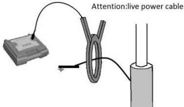
Fig.3.7 Clamp coupling method 2
