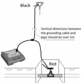
Fig.2.2 Direct connection mode wiring
