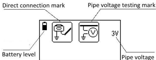
Fig.2.3 Pipe voltage measurement interface
