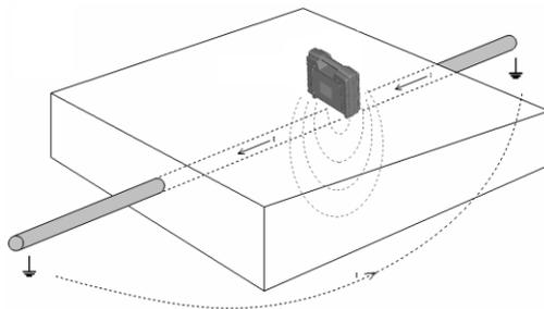
For pipe detection: this needs two people to cooperate for the detection, keep the Transmitter and Receiver at certain distance and move them simultaneously, they should have same direction. Please refer to page 17 Radiation detection.
