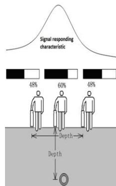
Fig.4.14 80% wide peak depth measurement
