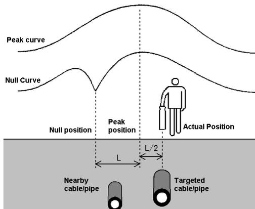
Fig.4.10 Positioning correction
