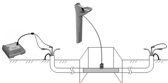
Fig.5.6 Sensor identification
