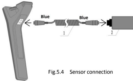
Fig.5.4 Sensor connection
