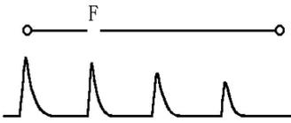
Fig.16-1 Left: break fault reflected waveform
