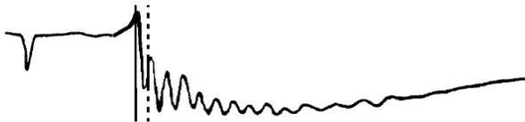
**C. Near distance Impact flash waveform**
