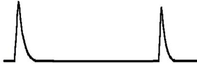
When the two waveform are displayed at the same time, obvious differences will appear at the fault point, and the fault distance can be easily judged and measured, as shown in Figure 31.
