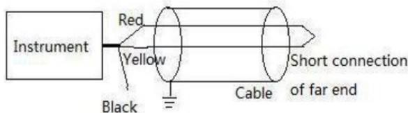
Figure 3.3.1 Connecting method of megameter
