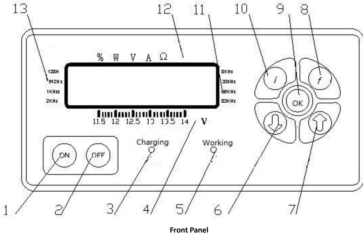
1&2.ON/OFF; 3.Charging Indicator; 4.Voltage Indicator; 5.Working Indicator; 6&7.Frequency Adjustment;
