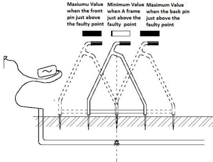
**Illustration of Positioning Fault Point using A Frame**
