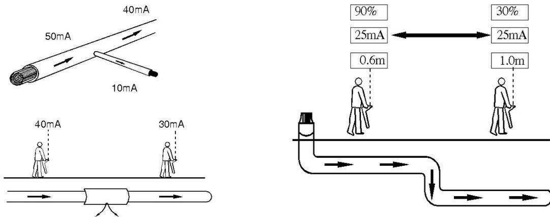
**Figure g: Tee and elbow at the current measurement diagram**
