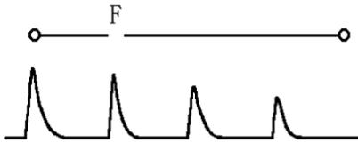
Figure 2A. Reflection waveform of disconnection fault
