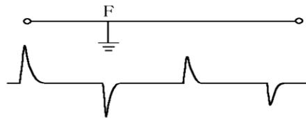
Figure 2B. Reflection waveform of cross fault
